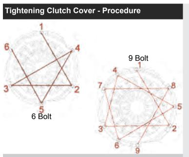
Slowly tighten the clutch cover bolts in a diagonal sequence When tight, torque to recommended specs in the same
