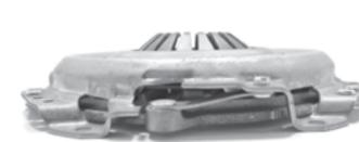
Clutch covers may differ between different manufacturers. When identifying the difference between samples it is important all variations in finger heights are benchmarked in the "installed" position. This is taken with the new clutch disc mounted and the clutch cover is torqued to the flywheel.
